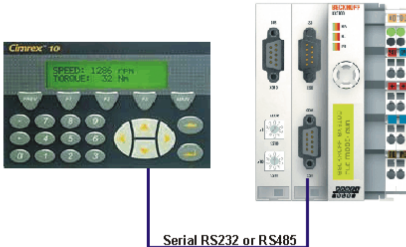
Fig. 108: Cimrex panel at the COM port of the BX controller
