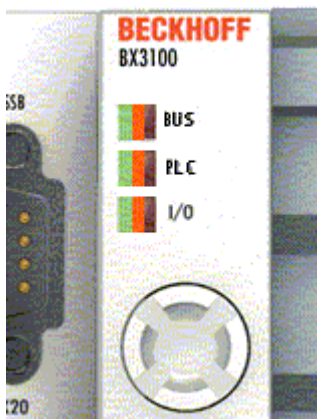
Fig. 125: Diagnostic LEDs for the PLC and the K-bus.
