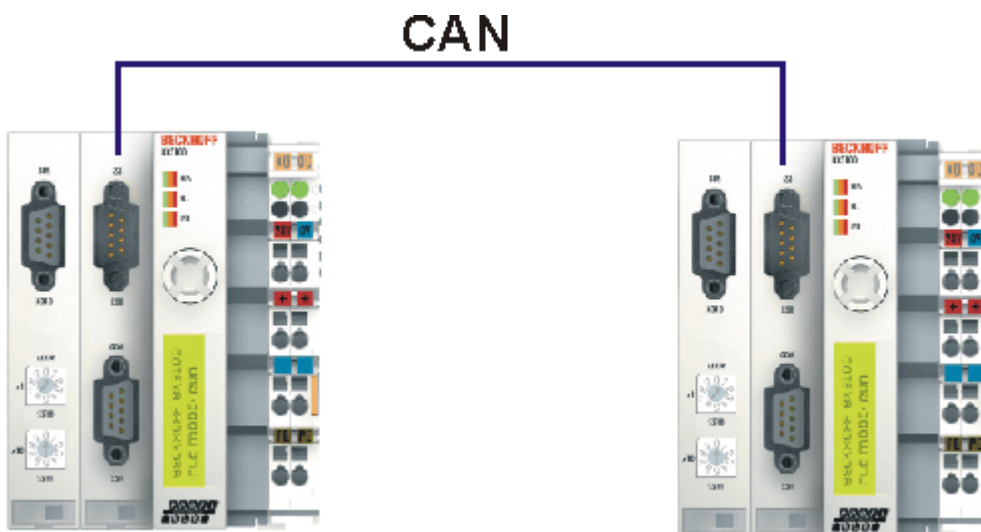
Fig. 59: Communication between BX controllers (via SSB)
