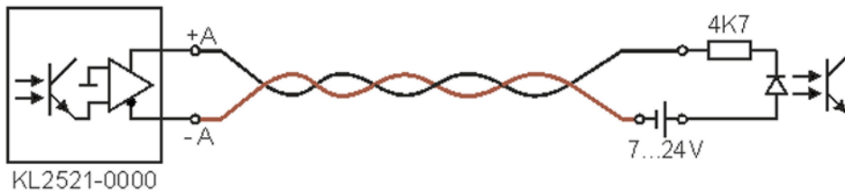
Fig. 15: KL2521-0000 up to hardware version 03 - wiring with external power source
