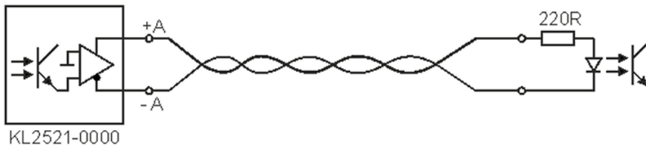
Fig. 14: EL2521-0000, direct connection to an optocoupler
