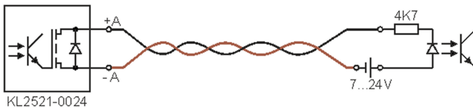
Fig. 16: KL2521-0024 - wiring with external power source
