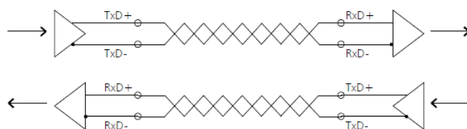
Fig. 3: Connection for RS422 transfer
