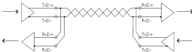
Fig. 2: Connection for RS485 transfer
