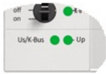
Fig. 9: Diagnostic LEDs at the front side
