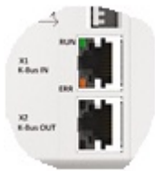
Fig. 10: Diagnostic LEDs at the rear side
