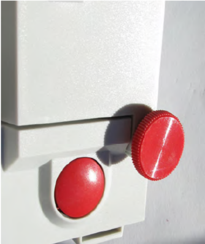
Fig. 54: Knurled screw of the SCT74xx
