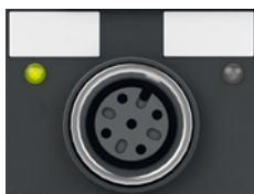
Fig. 28: Status LED on an M12 socket for EP1008-0022
