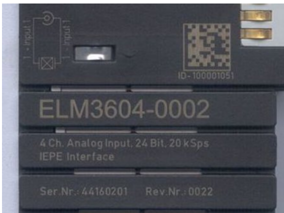
Fig. 26: ELM3604-0002 terminal with unique ID number (QR code) 100001051 and serial/ batch number 44160201
