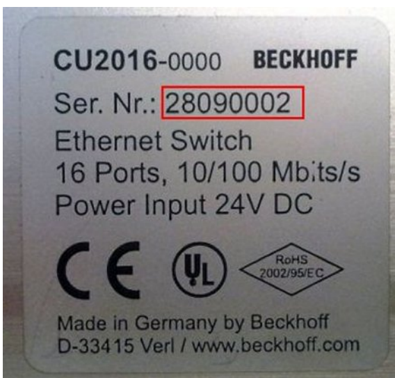
Fig. 21: CU2016 switch with serial/ batch number
