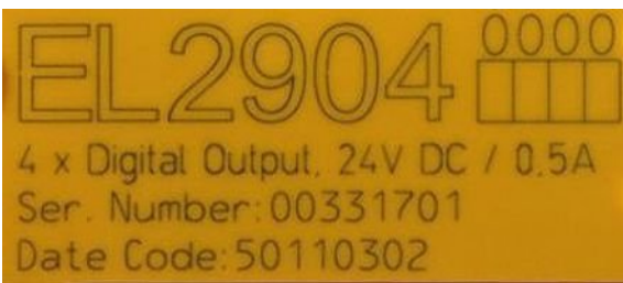
Fig. 31: EL2904 IP20 safety terminal with batch number/ date code 50110302 and unique serial number 00331701
