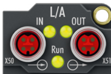
Fig. 5: Status LEDs for EtherCAT
