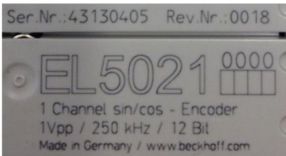
Fig. 4: EL5021 EL terminal, standard IP20 IO device with serial/ batch number and revision ID (since 2014/01)
