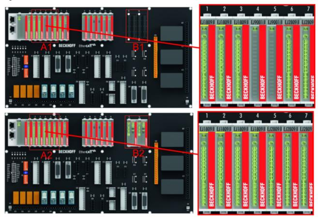
Fig. 22: Sample: Exchanging placeholder modules and assigning reserve slots
