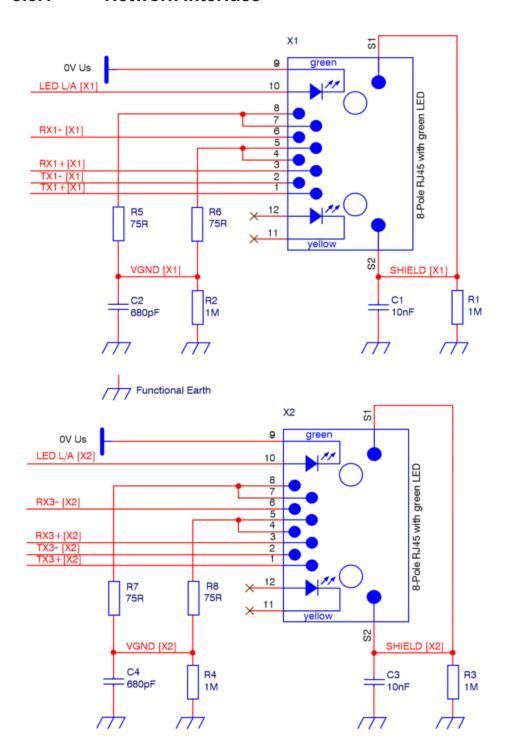
Fig. 9: Example schematic of a RJ45 based network interface
