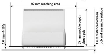
Fig. 15: Mounting distances EJ module - PCB
