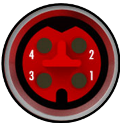
Fig. 30: Pin assignment M8, EtherCAT P In and EtherCAT P Out
