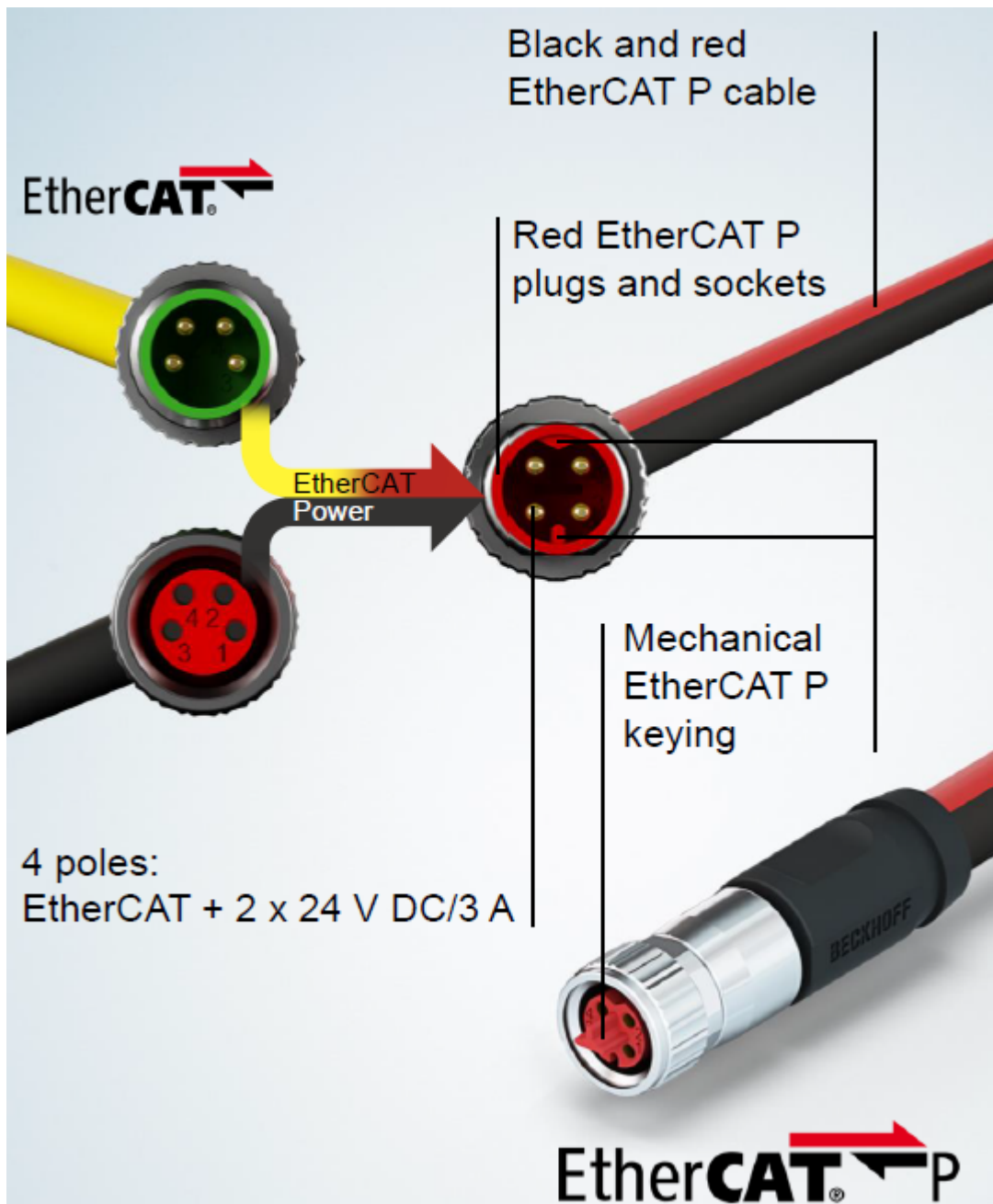
Fig. 15: Connector face: EtherCAT, Power and EtherCAT P
