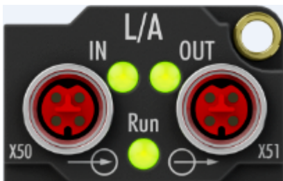
Fig. 29: EtherCAT-P-Box, Connectors for EtherCAT P
