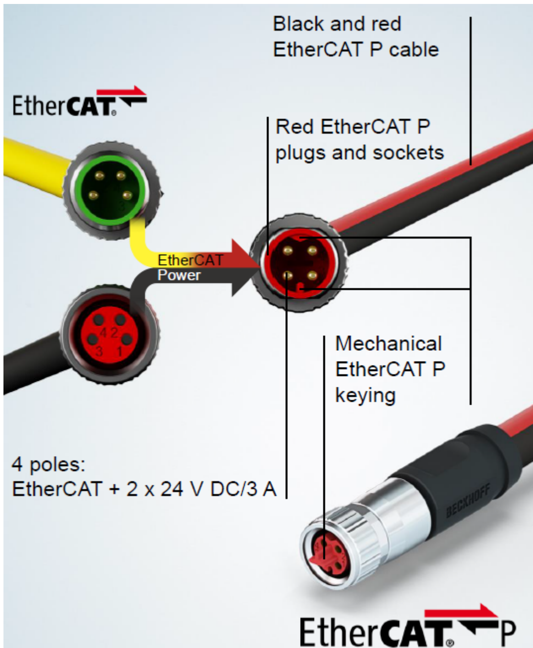
Fig. 15: Connector face: EtherCAT, Power and EtherCAT P
