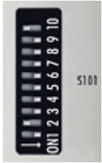
Abb. 15: DIP-Schalter S001: links off "0", rechts on "1"
