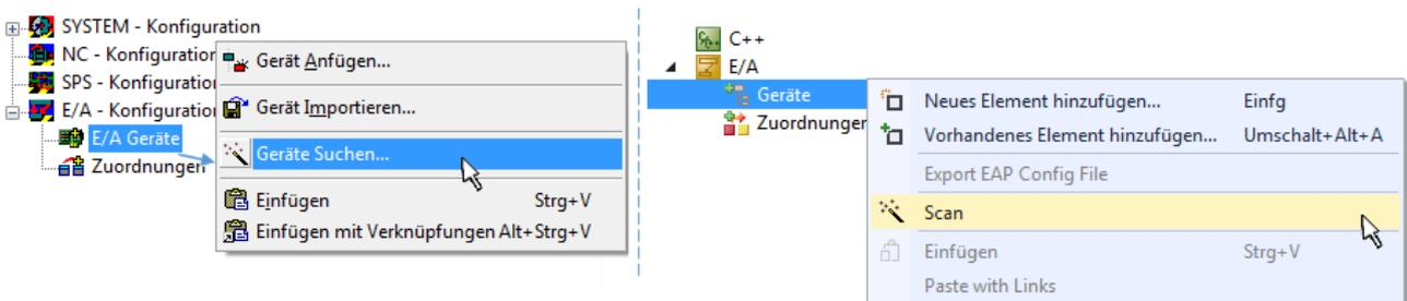
Abb. 90: Scan Devices (links: TwinCAT 2; rechts: TwinCAT 3)
