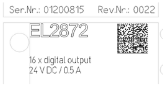
Fig. 1: EL2872 with revision 0022 and serial number 01200815
