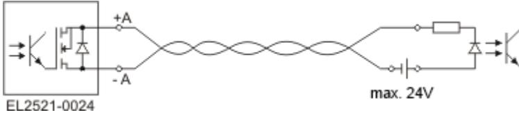
Fig. 27: EL2521-0x24, wiring with external power source
