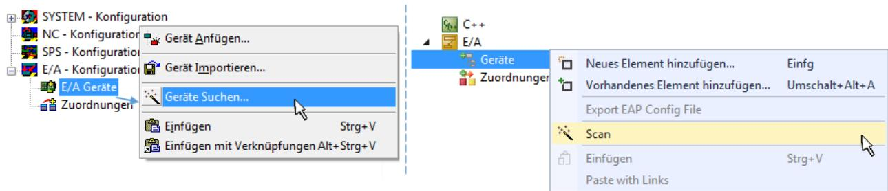
Abb. 102: Scan Devices (links: TwinCAT 2; rechts: TwinCAT 3)
