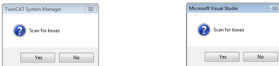
Fig. 149: Scan query after automatic creation of an EtherCAT device (left: TwinCAT 2; right: TwinCAT 3)
