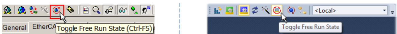
Fig. 184: TwinCAT can also be switched to this state by using a button (left: TwinCAT 2; right: TwinCAT 3)
