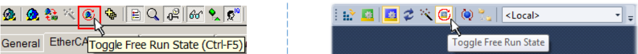
Fig. 111: TwinCAT can also be switched to this state by using a button (left: TwinCAT 2; right: TwinCAT 3)
