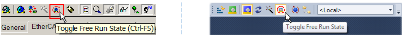
Fig. 109: TwinCAT can also be switched to this state by using a button (left: TwinCAT 2; right: TwinCAT 3)
