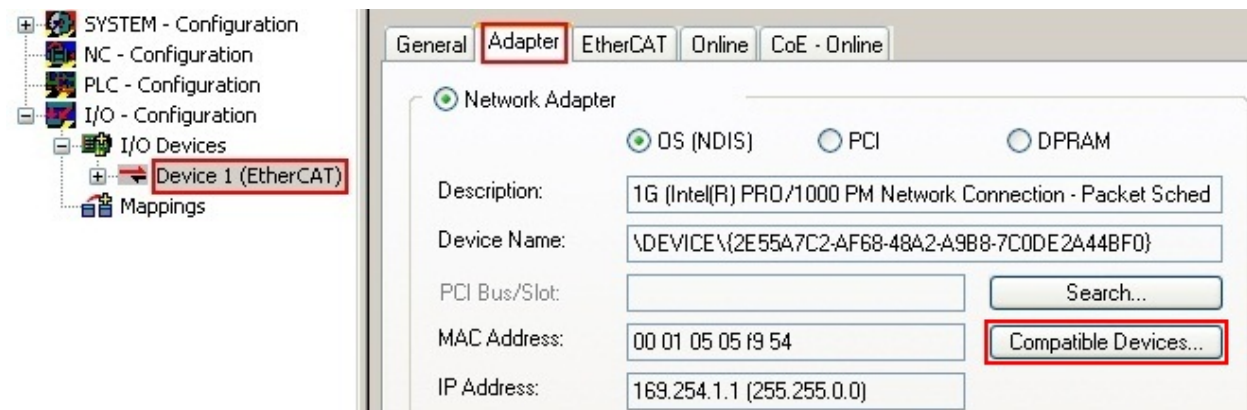
Fig. 74: EtherCAT device properties(TwinCAT 2): click on “Compatible Devices...” of tab “Adapte””
