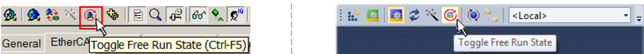
Fig. 122: TwinCAT can also be switched to this state by using a button (left: TwinCAT 2; right: TwinCAT 3)
