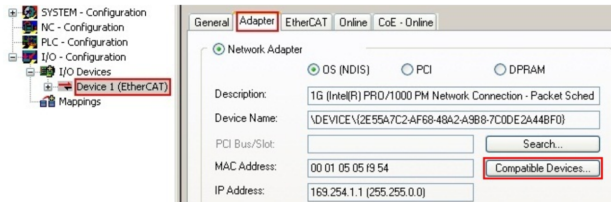
Fig. 87: EtherCAT device properties (TwinCAT 2): click on “Compatible Devices...” of tab “Adapter”
