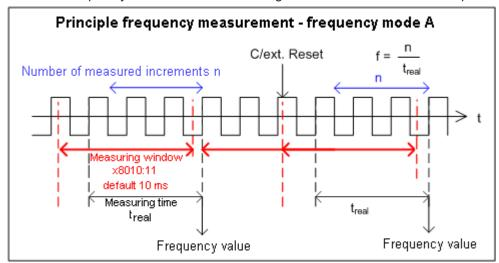
Fig. 147: Frequency measurement principle - frequency mode A
