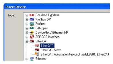
Fig. 92: Selecting the EtherCAT connection (TwinCAT 2.11, TwinCAT 3)
