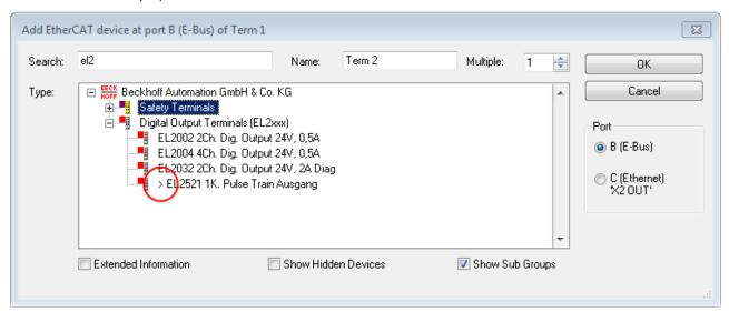
Fig. 87: Indication of an online recorded ESI of EL2521 as an example
