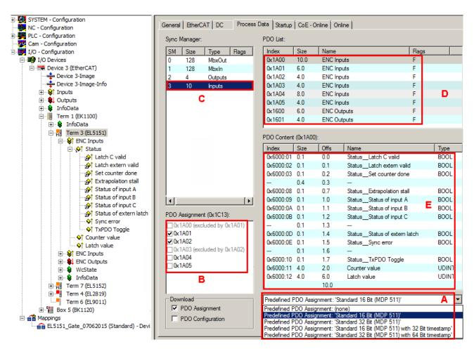
Fig. 144: Selection dialog "Predefined PDO Assignment", example of EL5151
