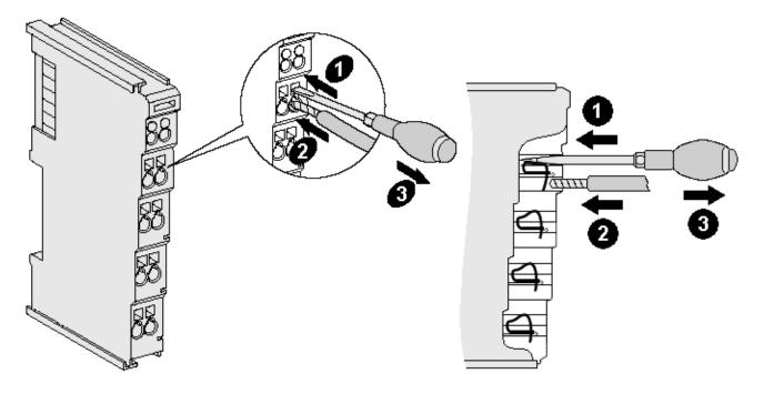
Fig. 24: Connecting a cable on a terminal point
