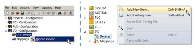
Fig. 91: Append EtherCAT device (left: TwinCAT 2; right: TwinCAT 3)
