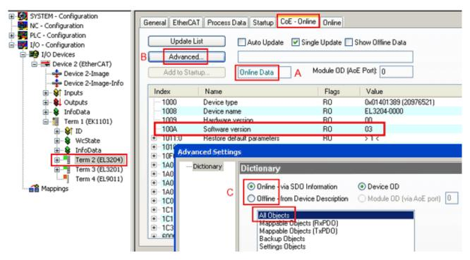
Fig. 183: Display of EL3204 firmware version
