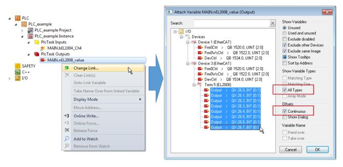
Fig. 67: Selecting several PDOs simultaneously: activate "Continuous" and "All types"
