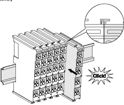
Fig. 18: Attaching on mounting rail
