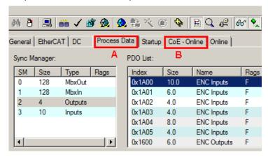
Fig. 143: Parameterization taking the EL5151 as an example
