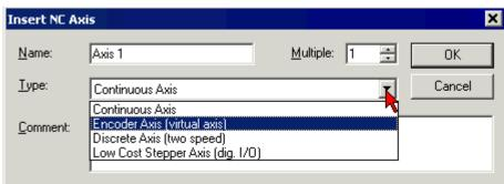
Fig. 170: Entering a name for the axis and selecting a type
