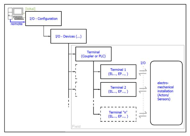
Fig. 32: Relationship between user side (commissioning) and installation
