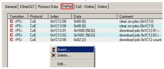
Fig. 14: Startup list in the TwinCAT System Manager
