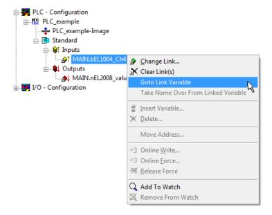
Fig. 48: Application of a "Goto Link Variable", using "MAIN.bEL1004\_Ch4" as an example
