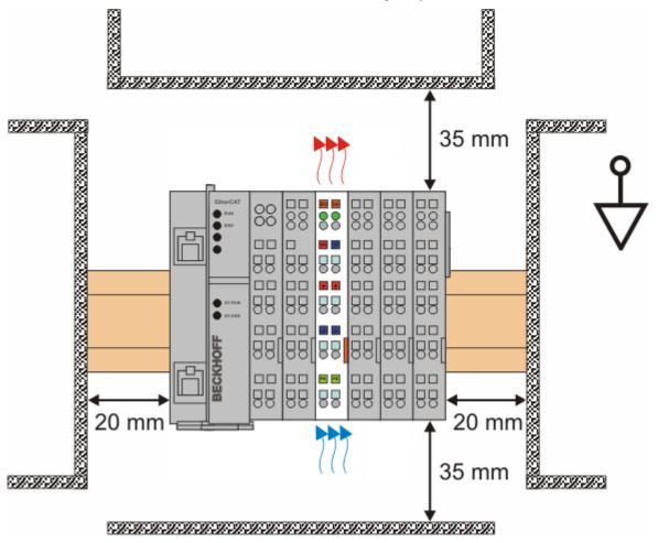
Fig. 25: Recommended distances for standard installation position
