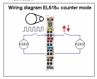
Fig. 154: Counter connection principle
