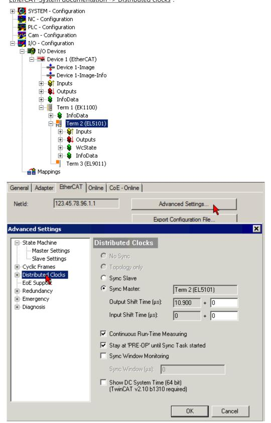
Fig. 176: EtherCAT Master, Advanced Settings, Distributed Clock
