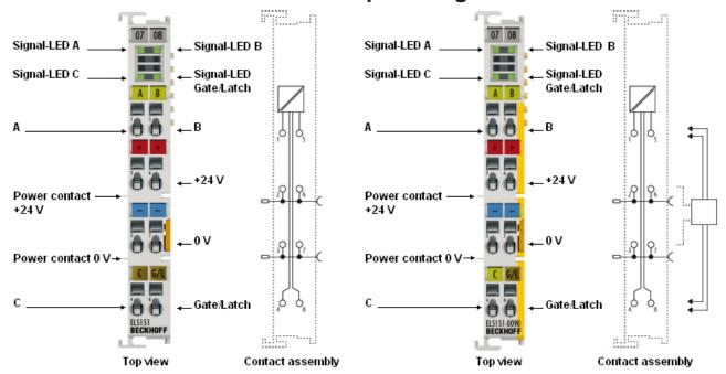
Fig. 29: EL5151, EL5151-0090 - LEDs and pin assignment
