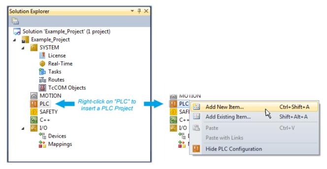
Fig. 60: Adding the programming environment in "PLC"
