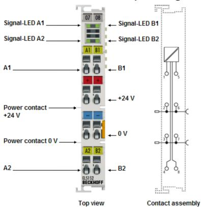
Fig. 31: EL5152 - LEDs and pin assignment
