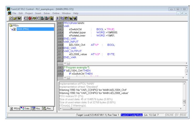
Fig. 42: Example program with variables after a compile process (without variable integration)
