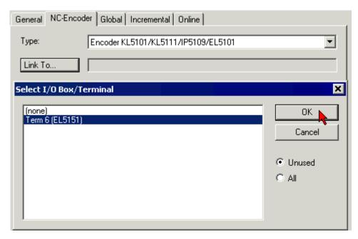
Fig. 172: Selecting and confirming an encoder terminal
