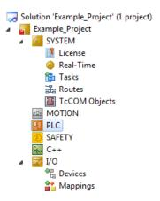
Fig. 53: New TwinCAT 3 project in the project folder explorer
