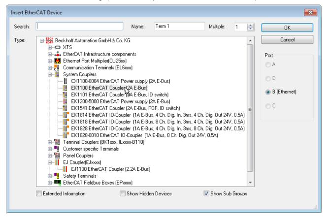
Fig. 96: Selection dialog for new EtherCAT device
