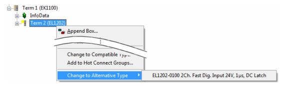
Fig. 121: TwinCAT 2 Dialog Change to Alternative Type
