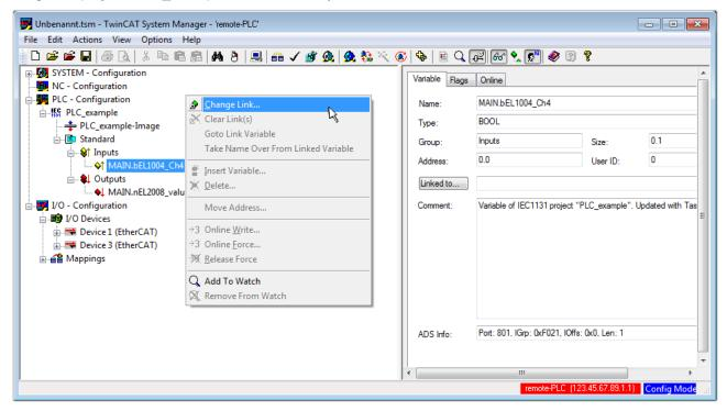
Fig. 45: Creating the links between PLC variables and process objects
