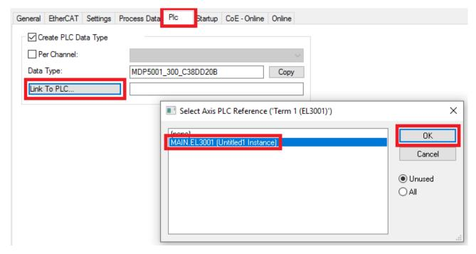
Fig. 71: Linking the structure
