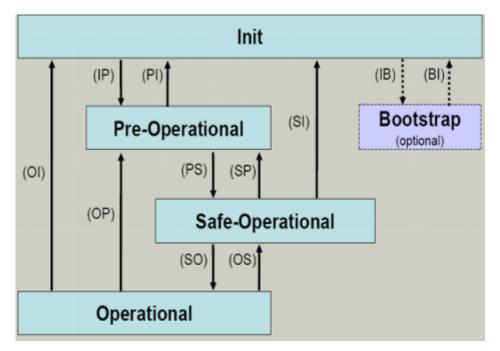
Fig. 12: States of the EtherCAT State Machine
