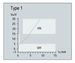
Fig. 9: Characteristic input 24 V<sub>DC</sub> type1
