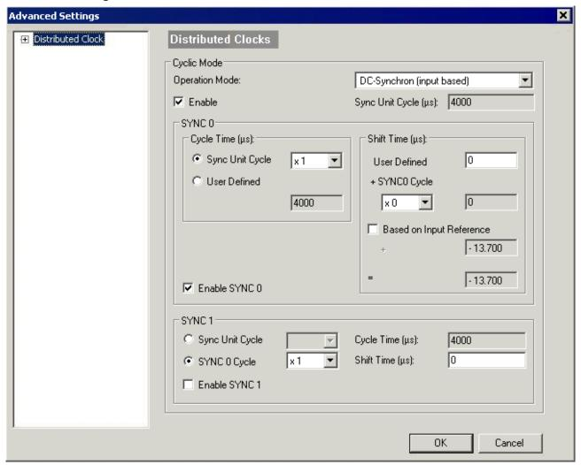
Fig. 175: Advanced Distributed Clock (DC) settings, EL51xx terminal
