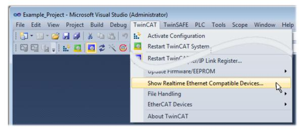
Fig. 75: Call up under VS Shell (TwinCAT 3)
