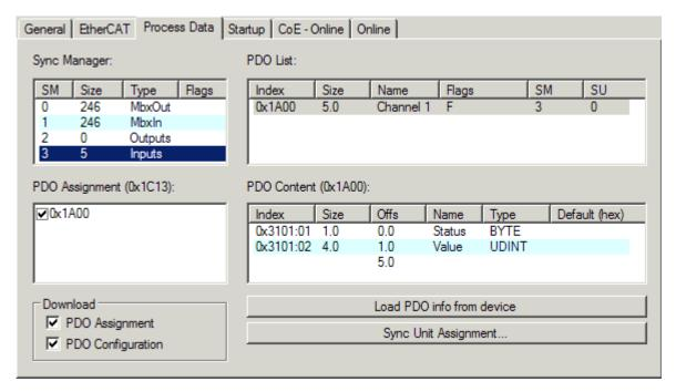
Fig. 125: "Process Data" tab
