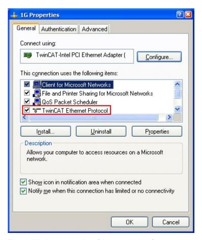
Fig. 79: Windows properties of the network interface
