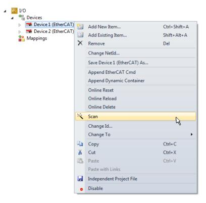
Fig. 59: Reading of individual terminals connected to a device
