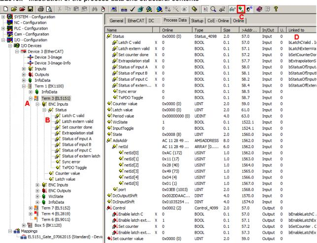
Fig. 141: Online illustration of the process data and structural contents in the System Manager, taking the EL5151 as an example
