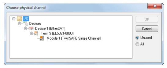
Fig. 161: Creating a link to TwinSAFE SC terminal
