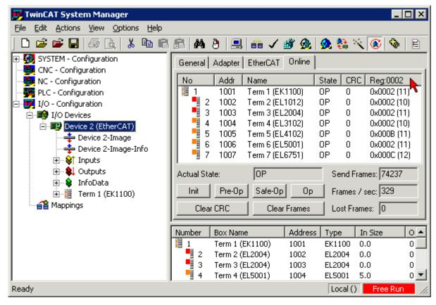
Fig. 185: FPGA firmware version definition
