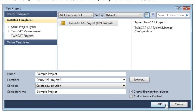
Fig. 52: Create new TwinCAT 3 project
