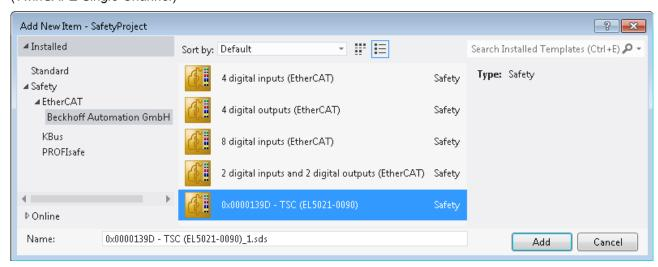
Fig. 160: Adding a TwinSAFE SC connection
