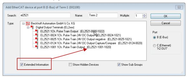
Fig. 97: Display of device revision
