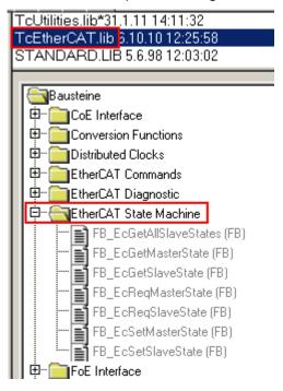
Fig. 138: PLC function blocks
