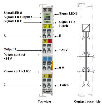
Fig. 30: EL5151-0021 - LEDs and pin assignment
