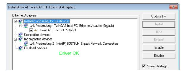
Fig. 80: Exemplary correct driver setting for the Ethernet port
