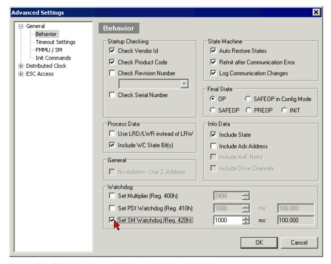
Fig. 11: eEtherCAT tab -> Advanced Settings -> Behavior -> Watchdog
