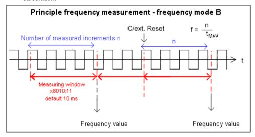
Fig. 148: Frequency measurement principle - frequency mode B
