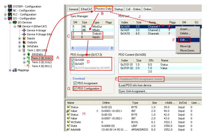
Fig. 126: Configuring the process data
