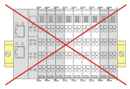
Fig. 28: Incorrect positioning
