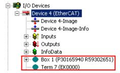
Fig. 115: Faulty identification
