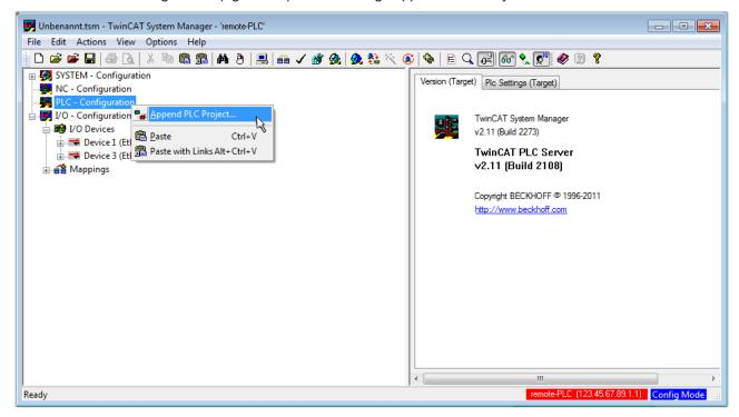
Fig. 43: Appending the TwinCAT PLC Control project
