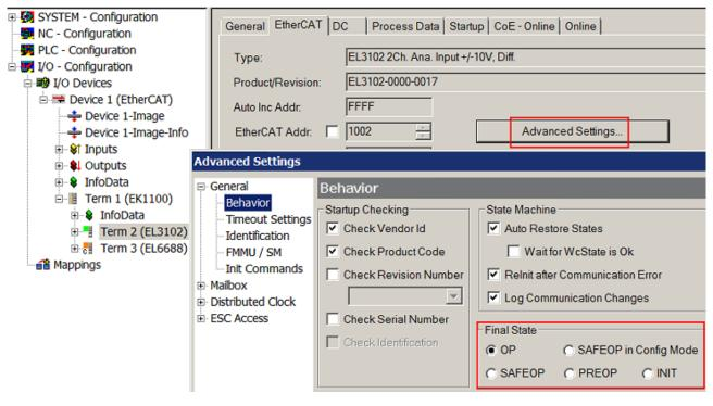
Fig. 137: Default target state in the Slave
