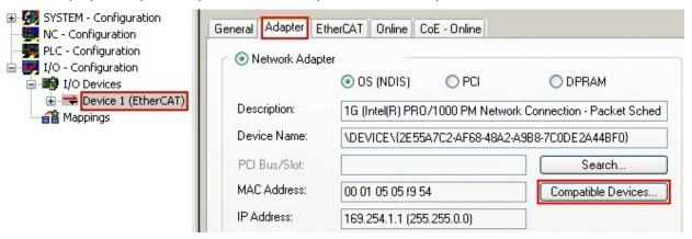
Fig. 78: EtherCAT device properties (TwinCAT 2): click on "Compatible Devices..." of tab "Adapter"
