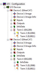
Fig. 39: Mapping of the configuration in the TwinCAT 2 System Manager
