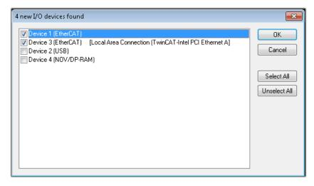
Fig. 57: Automatic detection of I/O devices: selection of the devices to be integrated
