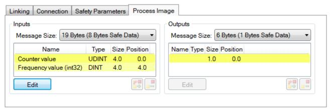
Fig. 163: Selecting the process data size and the process data
