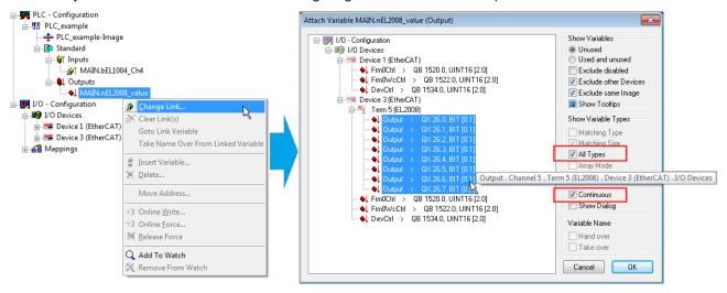
Fig. 47: Selecting several PDOs simultaneously: activate "Continuous" and "All types"
