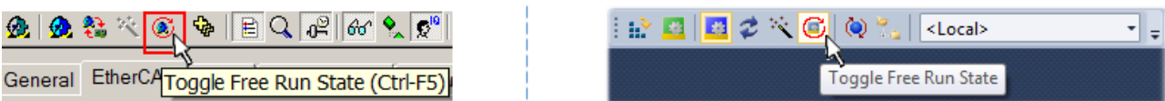
Fig. 113: TwinCAT can also be switched to this state by using a button (left: TwinCAT 2; right: TwinCAT 3)
