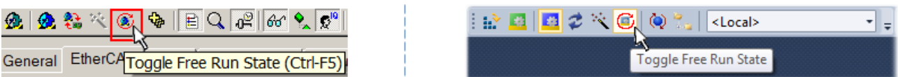
Fig. 97: TwinCAT can also be switched to this state by using a button (left: TwinCAT 2; right: TwinCAT 3)
