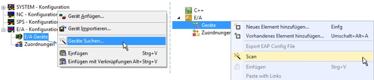
Abb. 43: Scan Devices (links: TwinCAT 2; rechts: TwinCAT 3)
