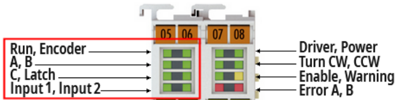
Fig. 39: EL7041-1000 LEDs (left prism)
