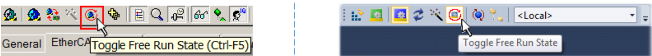
Fig. 129: TwinCAT can also be switched to this state by using a button (left: TwinCAT 2; right: TwinCAT 3)
