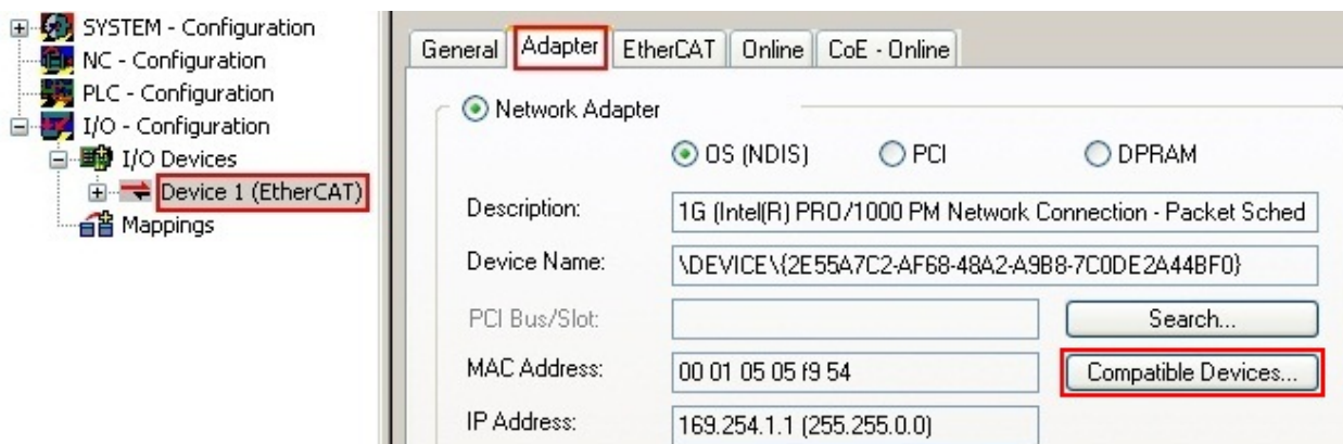
Fig. 84: EtherCAT device properties (TwinCAT 2): click on “Compatible Devices...” of tab “Adapter”
