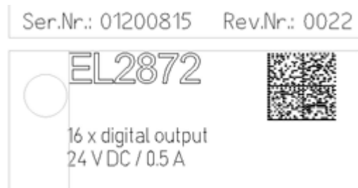
Fig. 1: EL2872 with revision 0022 and serial number 01200815
