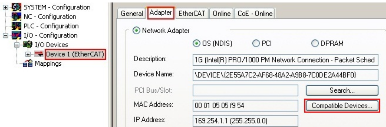
Fig. 275: EtherCAT device properties (TwinCAT 2): click on “Compatible Devices...” of tab “Adapter”
