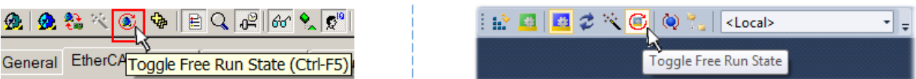
Fig. 310: TwinCAT can also be switched to this state by using a button (left: TwinCAT 2; right: TwinCAT 3)
