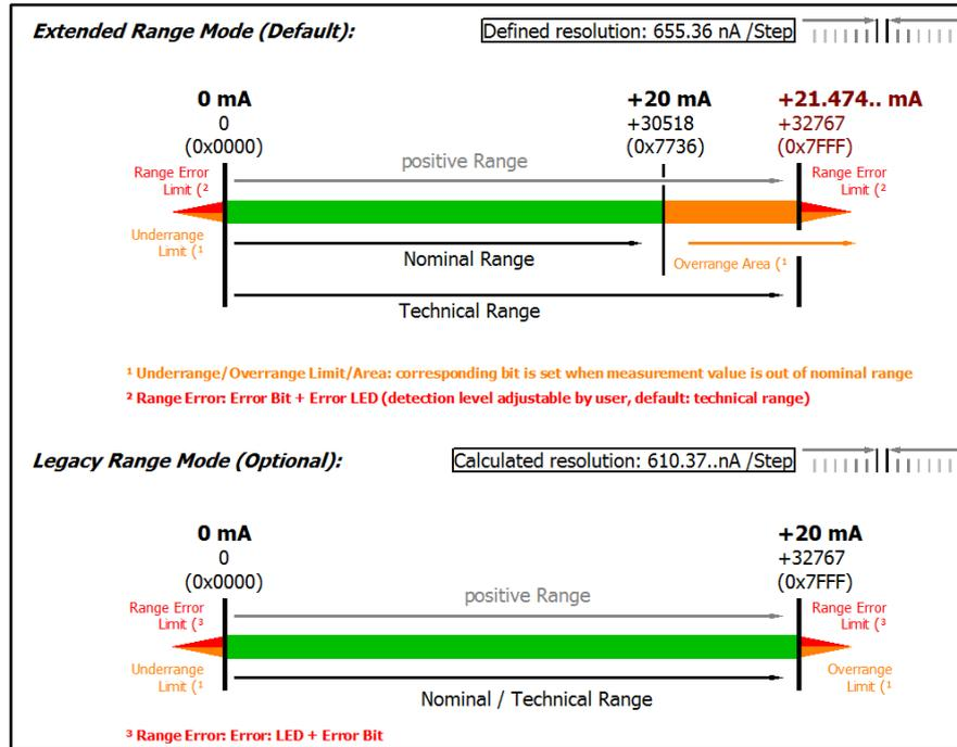
Technical note: The detection level for underrange and range error of 0 value area is located at -0.2 mA (-1% of the full scale value). This has been configured to prevent a misleading setting of the error bit. The process data value don't undercut 0x0000 then.
