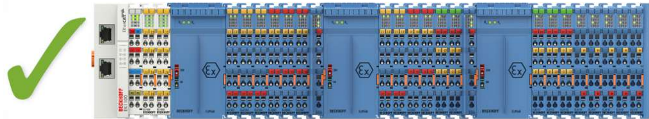
Fig. 8: Valid arrangement - multiple power supplies by ELX9560, each with an upstream ELX9410.
