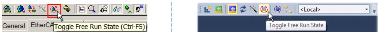
Fig. 101: TwinCAT can also be switched to this state by using a button (left: TwinCAT 2; right: TwinCAT 3)
