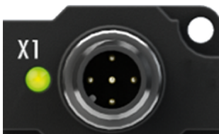
IO-Link Device Status LED (schmales Gehäuse)
