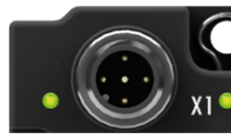
IO-Link Device Status LED (breites Gehäuse)
