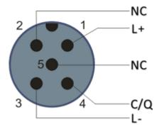
Fig. 7: Pin assignment Port Class A, Pin 2 not connected
