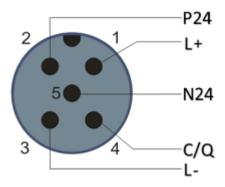
Fig. 9: Pin assignment Port Class B
