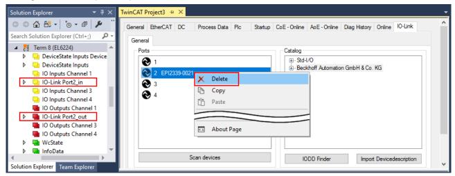
Fig. 28: Remove the device from port2
