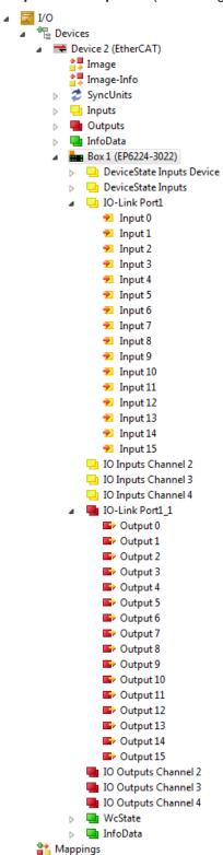
Fig. 4: EPI2339-002x Process image, digital inputs and digital outputs
