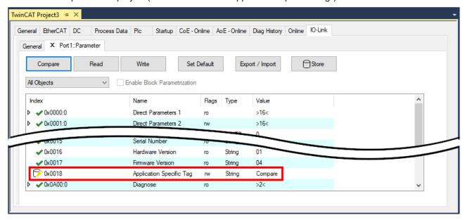
Fig. 33: Display of deviating data in the "Parameter" tab
