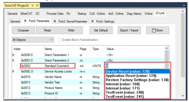
Fig. 42: Parameters IO-Link device "Standard Command"
