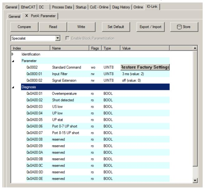
Fig. 48: IO-Link Device Parameter: showing Diagnosis EPI2339-0021 as example
