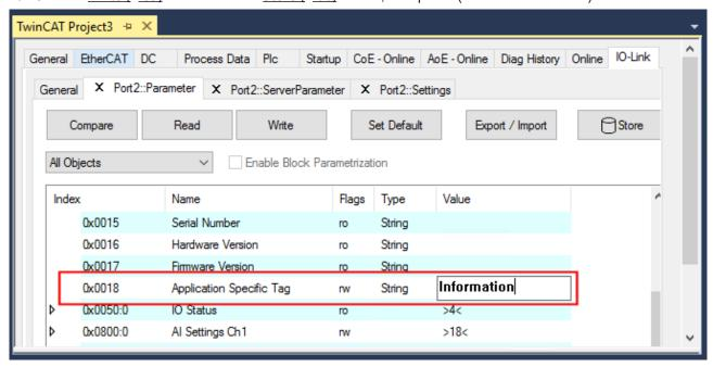
Fig. 43: Parameters IO-Link device: "Application Specific Tag"
