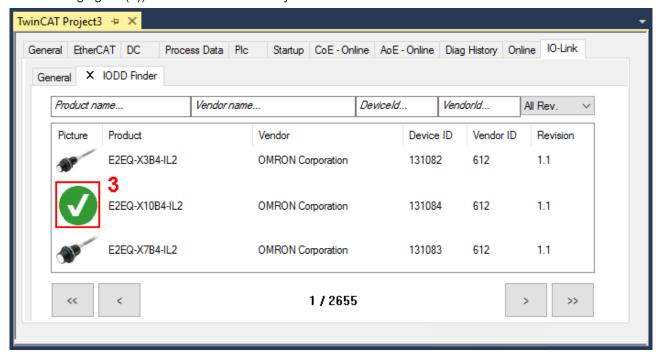
Fig. 21: IODD Finder, display of an already imported device description
