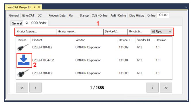
Fig. 20: IODD Finder, selection and import of the .xml-file
