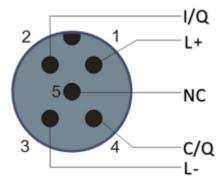
Fig. 8: Pin assignment Port Class A, Pin 2 connected
