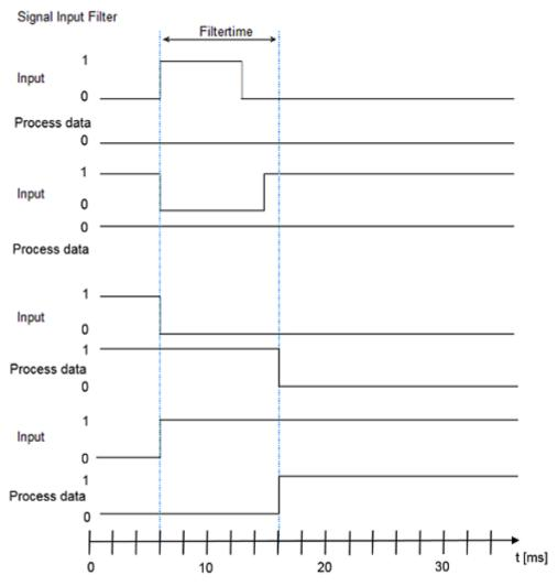
Fig. 49: Signal Input Filter
