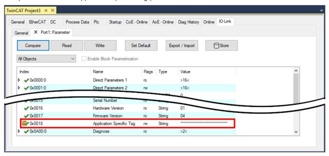
Fig. 32: Display of matching data in the "Parameter" tab
