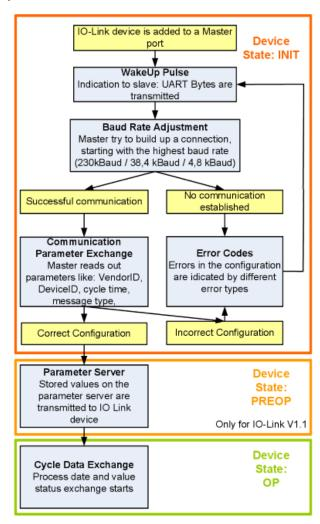
Fig. 5: Establishment of IO Link communication
