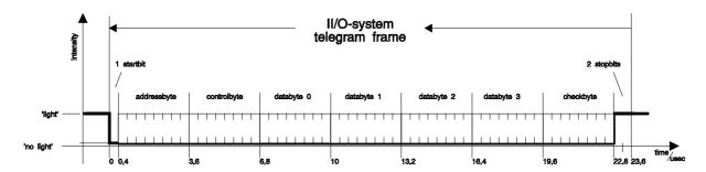
picture 2: Telegram structure of the II/O-System
