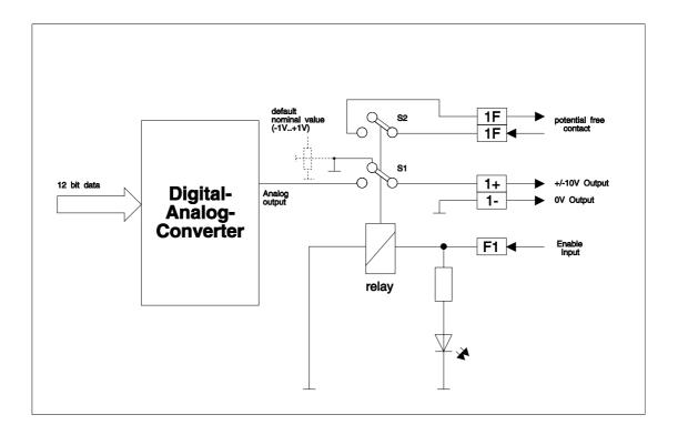
In order to take the analog voltages from the connections, the appropriate relay of a certain analog channel has to be selected by applying 24 VDC to the relay input F1..F4 (connector X22).
