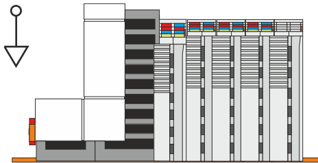
Fig. 8: Embedded PC CX8180, horizontal installation position.
