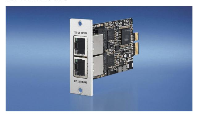
Beckhoff PCIe modules are based on a new definition of highly integrated PCI Express plug-in cards and follow the trend towards ever smaller PCs. The function of PC plug-in cards is integrated in a compact format that is suitable for harsh industrial environments.
