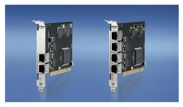
Up to four Ethernet channels in one slot: The Ethernet PCI network cards from Beckhoff save space and costs. They can be used in office and automation networks and offer the following benefits:
