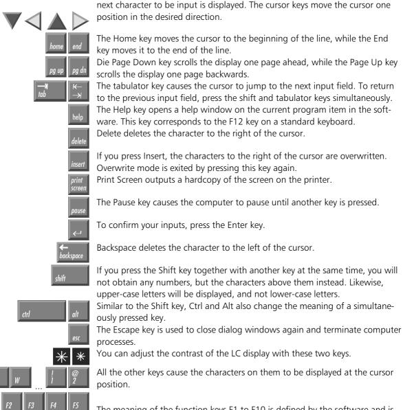
The meaning of the function keys F1 to F10 is defined by the software and is displayed at the bottom margin of the display.
