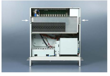
Remove the 2 fastening screws of the card holder (see arrows) using a cross-head screwdriver. The holder can then be lifted up.
