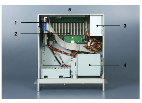
A plug-in motherboard (1) and a 14-slot passive backplane (2) are located under the housing cover.
