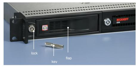
The hard disks are located into two removable hard drive racks at the front of the Industrial PC. After unlocking the flaps of the removable racks you can swivel out the hard disks. Now the disks can be removed.
