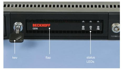
The control elements are located behind a flap at the front side of the Industrial PC. After unlocking the flap with the key it can be folded down. You now have access to the control elements:
