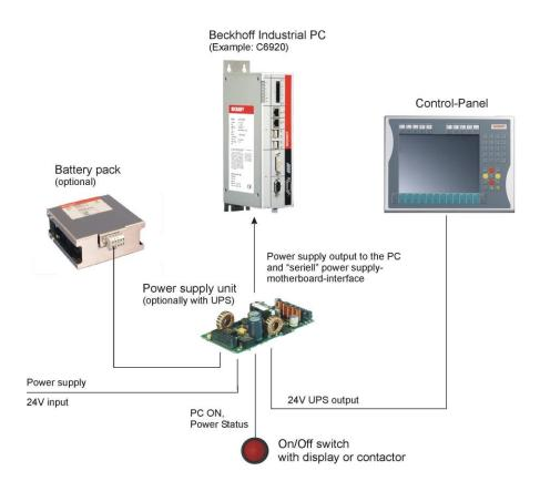
Industrial PCs equipped with a UPS are in actual use frequently switched off by simply turning off the supply voltage. In this case the PC shuts down via the battery. However, over time this reduces the service life of the battery.
