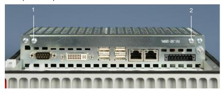
After loosening the two screws (1) and (2) the cover plate can be removed.
