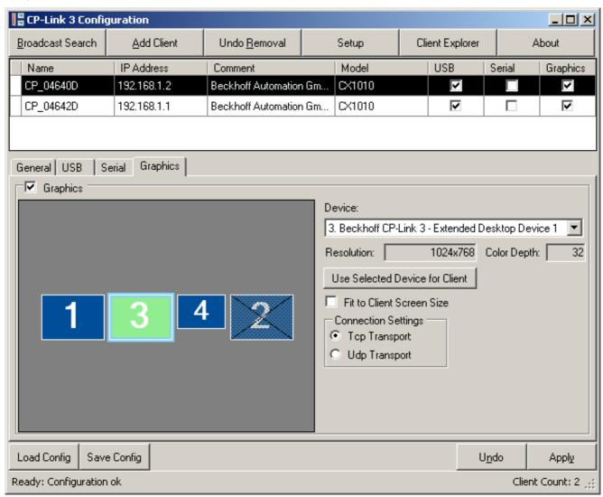
The "Virtual Graphics" functionality for the client can be enabled or disabled by setting or clearing the tick in the *Graphics* selection box.
