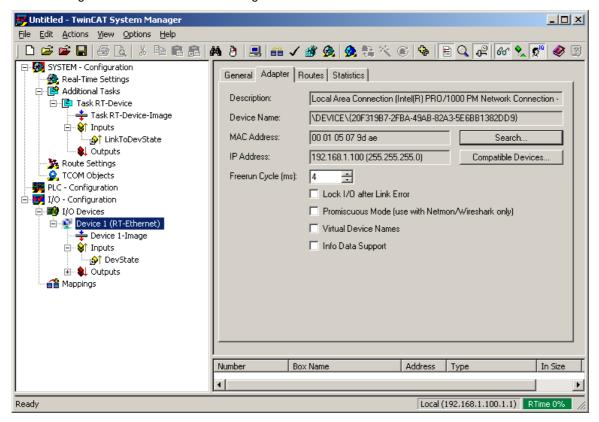
The following illustration shows an I/O Configuration for a client with one RT Ethernet device:
