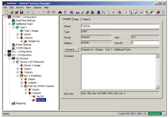
One or more network variable(s) are added to the client Subscriber corresponding with the network variables configured on the host PC. In the dialog window which appears, after the Publisher computer has been searched for, a list of all Publisher variables is displayed and the corresponding variable can be added to the Subscriber.
