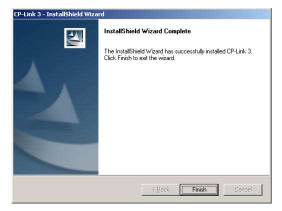
Click *Finish* in order to terminate the installation process. After the installation the operating system needs to be restarted. The necessary software components have now been installed on your computer, and a link to the CP-Link 3 configuration application placed on the desktop.
