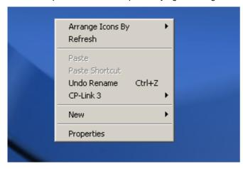
If the mouse is pulled to the CP-Link 3 entry, a window opens showing a list of all the open windows currently displayed on the host computer.
