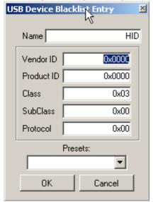
Hexadecimal notation (in which 0x can be omitted) is typically used for the entries in these fields. It is also possible to select a predefined class of devices (e.g. *Mass Storage*), and to enter this into one of the lists.
