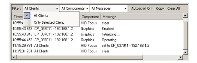
Filtering on messages of certain components: The messages of the selected components are shown. By default the messages of all components are shown.
