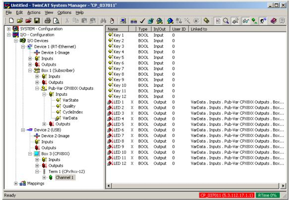
The cycle time of the RT Ethernet device defines the cycle time for data exchange with the Bus Coupler. The recommended cycle time for data exchange with the terminals at the Bus Coupler is between 50 and 80 ms (see also
