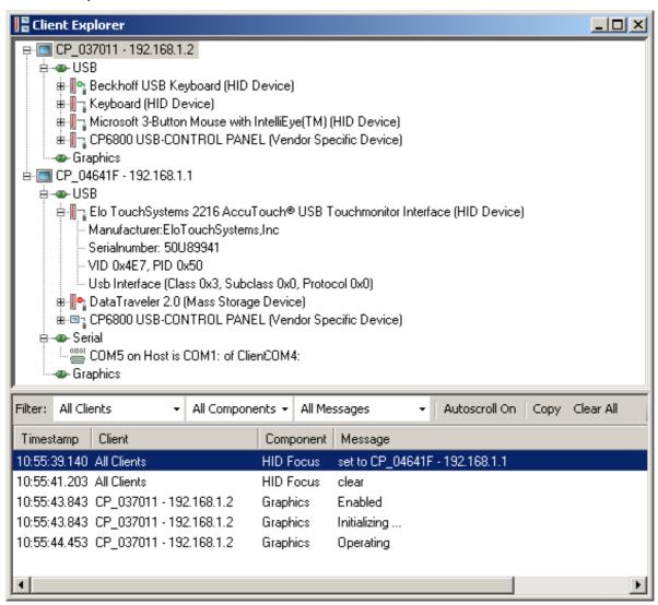
The upper section pictures a tree structure, which on one side shows the currently activated CP-Link 3 Configuration and on the other contains current status information. In the lower section is a message window in which warnings, error messages and status information is given in the form of text.
