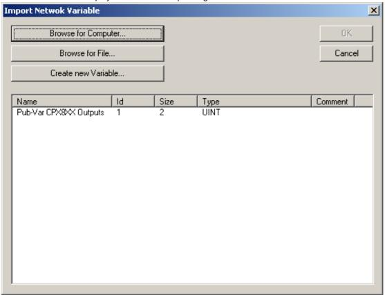
The client network variable now can be linked with the output variables of the Bus Coupler.
