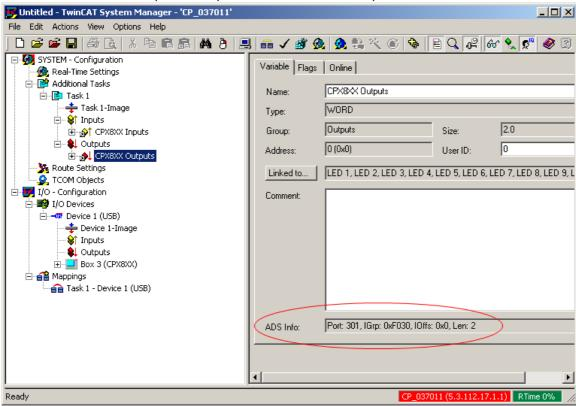
The "ADS Info" of the client task variables are then used for ADS communication in the host PC PLC program.
