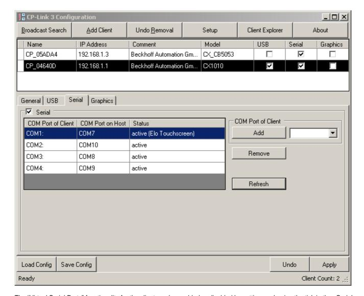
The "Virtual Serial Ports" functionality for the client can be enabled or disabled by setting or clearing the tick in the Serial selection box.
