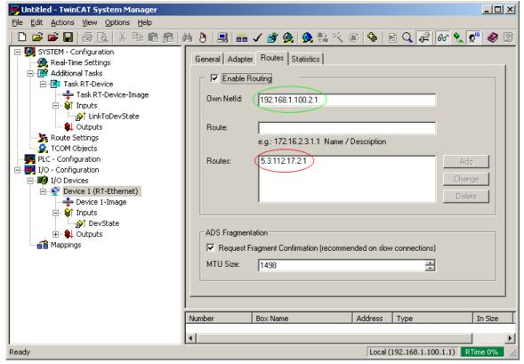
The NetId of the host PC RT Ethernet adapter is added to the client "Routes" table:
