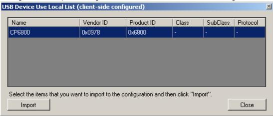
By using the *Import* button the selected client-side configured Use Local List entries are being adopted to the list configured on the host PC.
