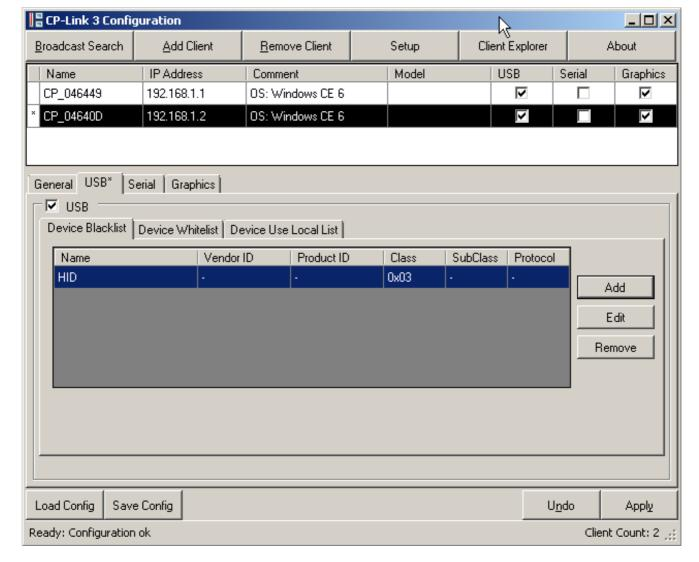
The "Virtual USB" functionality for the client can be enabled or disabled by setting or clearing the tick in the USB selection box.
