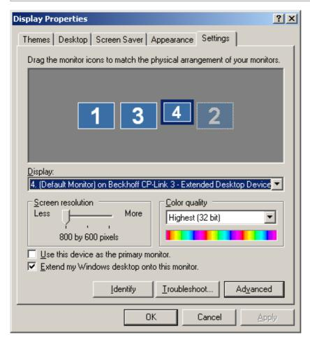
The display device is selected by clicking on the corresponding monitor symbol, and this can be seen from the border. The settings for the selected display device can now be modified in the lower part of this dialog.
