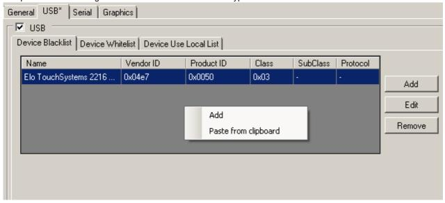
Filters for USB devices can be added or removed through the *Add* and *Remove* buttons. Clicking the *Edit* button allows filters that have already been created to be edited. Alternatively, you can use the context menu to add, remove or edit filter entries. In addition you can use the context menu to paste an entry from the clipboard if you previously copied an entry to the clipboard using the Client Explorer (see also the Client Explorer section).
