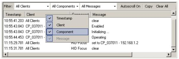
Above the output field are several selection boxes which allow different filters to be defined. These filters determine which messages are shown or not shown in the output field. Filtering can be done using any combination of the following criteria:
