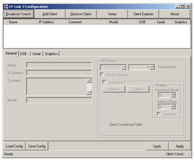
Clients can be added to the client list by clicking *Broadcast Search* or on *Add Client*. Clients can be removed from the client list with a click on *Remove Client*.
