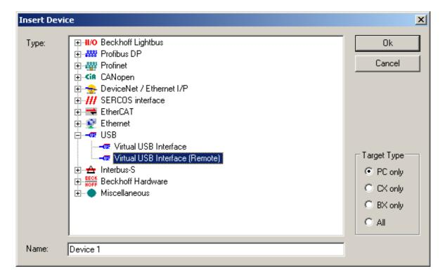
After the device has been added the NetID of the target system can be defined on the "Remote" tab. This can either be entered directly or also determined by the "Choose Target" button. When the target system has been reached then connected boxes can be addressed and configured as usual. The recommended cycle time for data exchange with the terminals at the Bus Coupler is still between 50 and 80 ms (see also cycle time for data exchange).
