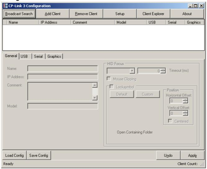
The client list, which is still empty, is located in the upper part of the configuration interface, while the settings for marked clients will later be listed in the lower part.
