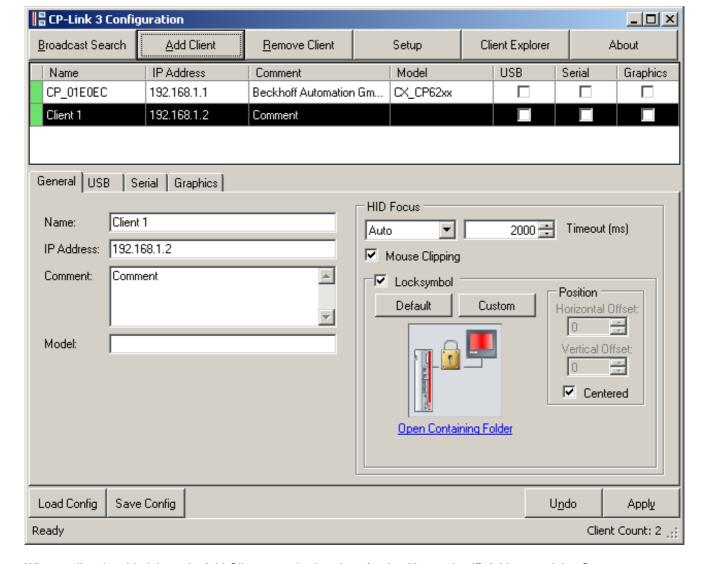
When a client is added through *Add Client*, standard settings for the *Name*, the *IP Address* and the *Comment* are loaded. These settings may need to be modified.
