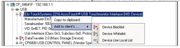
If you copy the device information into the clipboard ( *Copy to clipboard* ) you can paste the copied information in the configuration window in order to create a device filter entry (see also the Client Configuration section - Edit USB device filters).
