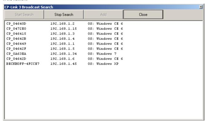
The desired device can be added by clicking the Add button or by double-clicking, and will then appear in the client list.
