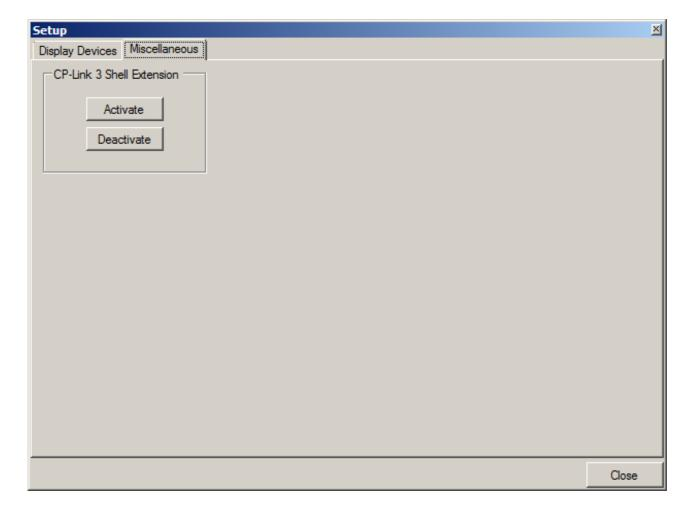
The CP-Link 3 Shell Extension can be switched on or off in the *CP-Link 3 Shell Extension* area. The CP-Link 3 Shell Extension is used to extend the desktop context menu (see also the CP-Link 3 Shell Extension section).
