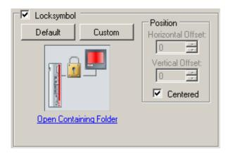
By clearing the tick in the *Centered* selection box a vertical and horizontal offset can be specified by using the *Horizontal Offset* and *Vertical Offset* fields. The offset's origin is the upper left corner of the host display's screen content shown on the client.
