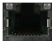
RJ-45 connector (Ethernet 10/ 100 MBit)
