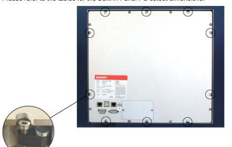
Release clamping levers,
