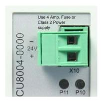
The USB hub CU8004-0000 requires a 24  $V_{DC}$  supply for it's operation. The connection is made by means of the terminal X10, labeled 24 V. This supply feeds the hub electronics and, over the USB downstream ports, the connected USB devices (5  $V_{DC}$ ). It is protected against polarity reversal.
