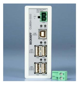
The CU8004-0000 Beckhoff USB hub offers 4 USB downstream ports (type A). It can be used universally in automation and office applications. The hub meets the special requirements of industrial applications through several outstanding features:
