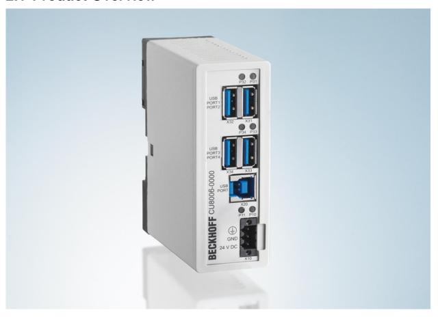
The CU8006 DIN rail-mount USB hub has four ports and supports the USB 3.0 data transfer rate of up to 5 Gbit/s, but is also compatible with slower USB standards. USB 3.0 devices can be connected at a distance of up to 3 m. Connection to USB 1.1/ USB 2.0 devices is possible with 5-m cables.
